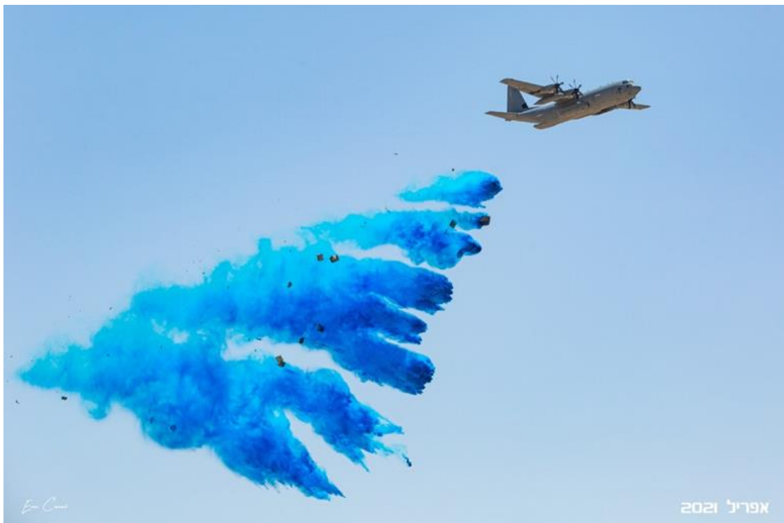
Figure 160. An experiment of dropping flame retardants using the Hercules aircraft.
