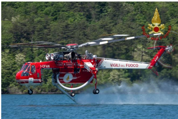
Figure 36. The Erickson S64 during the scoop with the sea snorkel.
