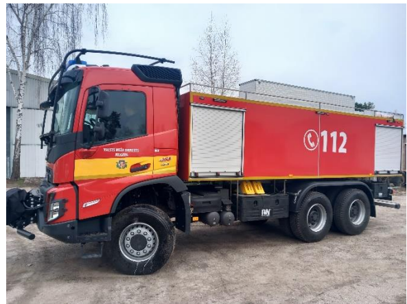
Figure 49. Volvo FMX 6X6 tanker truck.
